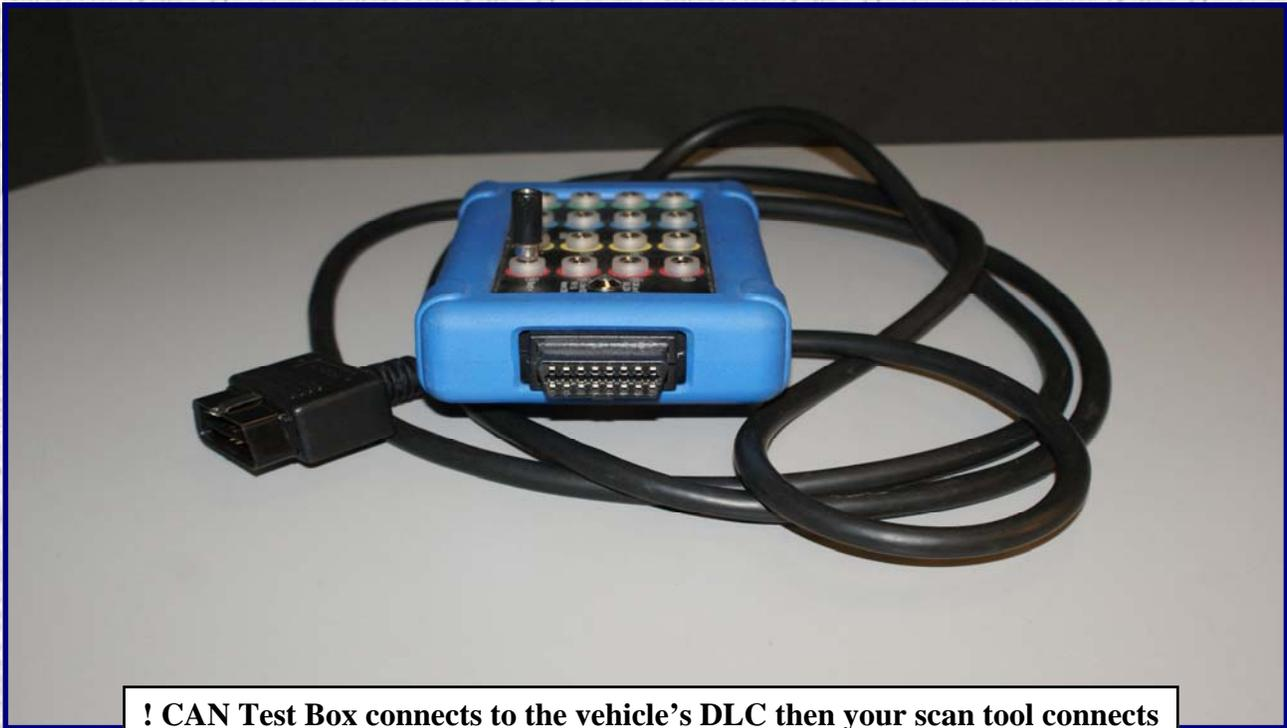
**! CAN Test Box connects to the vehicle's DLC then your scan tool connects to the DLC plug on the CTB....A very nifty tool for troubleshooting!**
