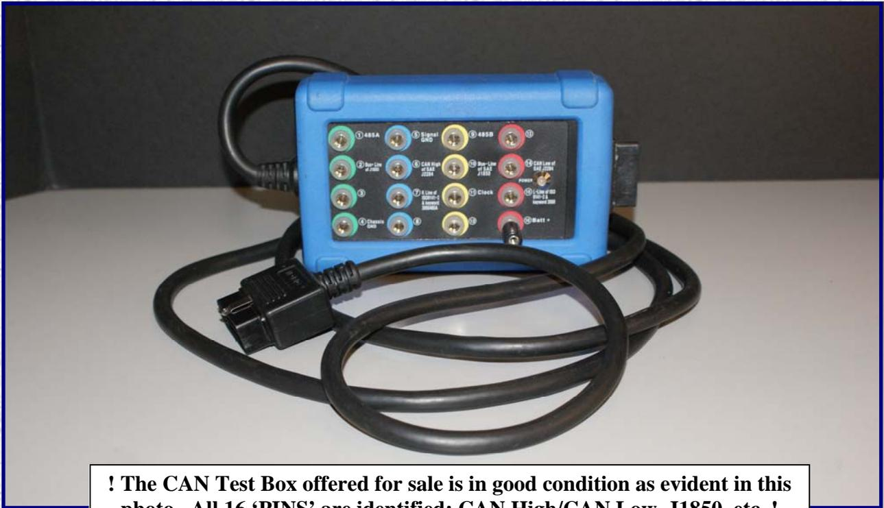
**! The CAN Test Box offered for sale is in good condition as evident in this photo...All 16 'PINS' are identified: CAN High/CAN Low, J1850, etc. !**
