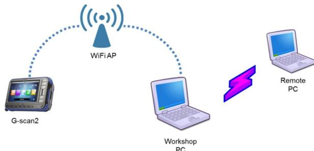
Remote Control mode can be activated by pressing F2 and F5 keys together from the main menu.
