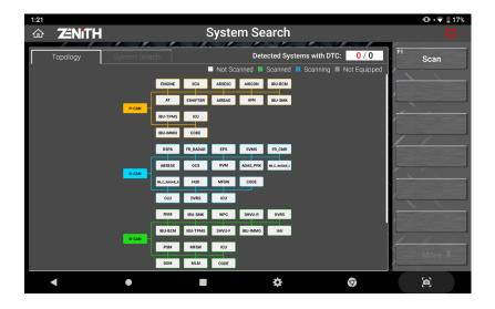
The Topology function supported by Zenith Z5 visualizes the structure and hierarchy of the in-vehicle network control modules and check the fault codes of each system (Z5 Only).
